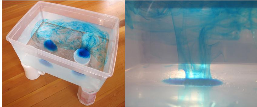
5. Explanation: The hot water in the styrofoam cup heats up the water and food dye directly above it, making this region flow upwards in the water (because it is less dense than the surrounding cooler water). It takes heat energy with them, and is moving by “convection”. The visualized convection currents are beautiful as they trace out the curving patterns of heated water.
